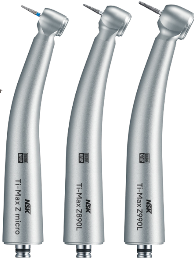
Micro Head Power : 20 W Speed : 380,000-450,000 min -1 Head Size : ø9.0 x H 10.8 mm Miniature Head Power : 41 W Speed : 320,000-400,000 min -1 Head Size : ø10.6 x H 10.8 mm Standard Head Power : 44 W Speed : 280,000-360,000 min -1 Head Size : ø12.1 x H 12.7 mm
